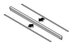
Don't bend or discard the stiffeners. You need to use them again. 5. Carefully insert the new blade rubber. Then install the blade assembly in the reverse order of removal.
